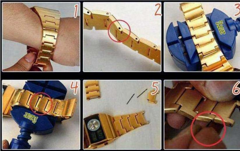
**NOTE:** the engraved arrow on the backside of the bracelet showing the direction in which the link pin should be pushed and lay the bracelet in the cradle as shown above. Align the pin of the pin pusher with the link pin, being careful to center it. Once centered, apply slight pressure until you feel the pin begin to move and then turn fixture upright as shown in illustration. This slight pressure will keep the pin pusher in alignment with the link pin while the tool is being turned upright.
