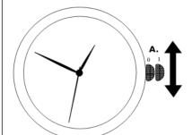
1. Pull the crown out to position "1" (part A) which will allow you to position watch hands for proper time selection. Once time is set, push crown back into original "o" (zero) position.
