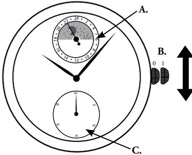
1. Pull the crown (part B) out to position "1" and rotate it to the desired time.
